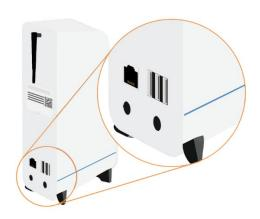
2. Rotate the Wi-Fi antenna on the back of the DASH® Instrument clockwise so that it is facing straight up. Tighten the knob next to the Instrument if needed to hold it firmly in place.
