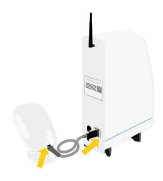
4. Connect the DASH® Instrument's power adapter to the round socket on the back of the DASH Instrument. The flat side of the plug should be up.
