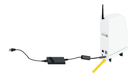
5. Connect the power cord to the adapter, then plug power cord into 120VAC outlet.
