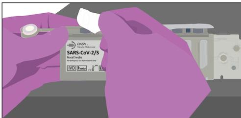
**4.6.2** Insert Swab into specimen chamber, which is the opening closest to the cap.
