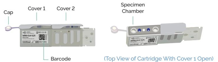
**3.5.1** First, Place Cartridge on flat surface and peel off Cover #1. DO NOT flip Cartridge over after peeling off Cover #1, as this part of the Cartridge has liquid in it.
