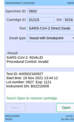
NOTE: The test results will be displayed on the DASH Analyzer touchscreen and printed after the test has been completed. The Procedural Control will display Valid on the results screen in a SARS-CoV-2 negative sample or SARS-CoV-2 positive sample. The Procedural Control is Valid if it meets the validated acceptance criteria. Screenshots of potential results screens are shown above, and the possible test results are summarized in the Table of Test Results and Interpretations below.
